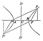
Through C, the middle point of F'F, draw CD perpendicular to F'F, and let C be the origin of a system of rectangular co-ordinates, of which AB, DD' are the axes. Let x and y represent the co-ordinates of the point P.
